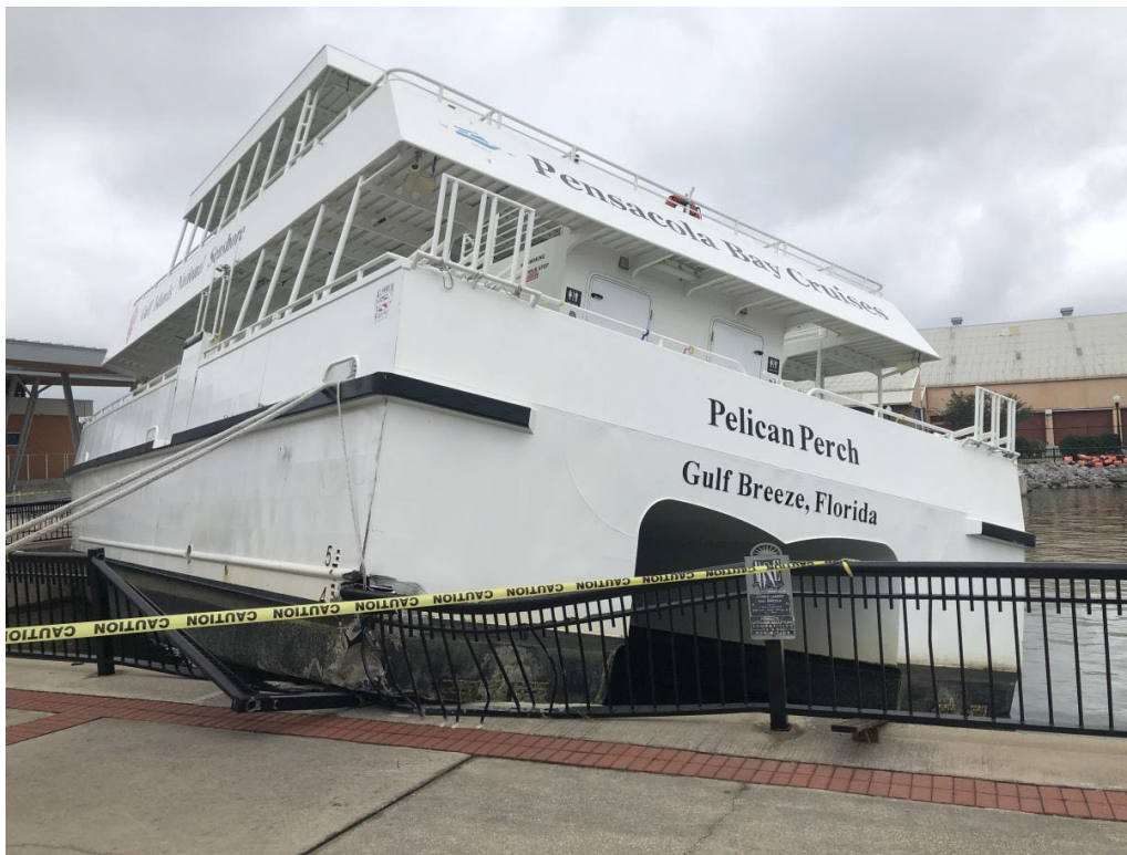
Figure 7: Damage to Pensacola Bay Ferry from Hurricane Sally's storm surge 25
