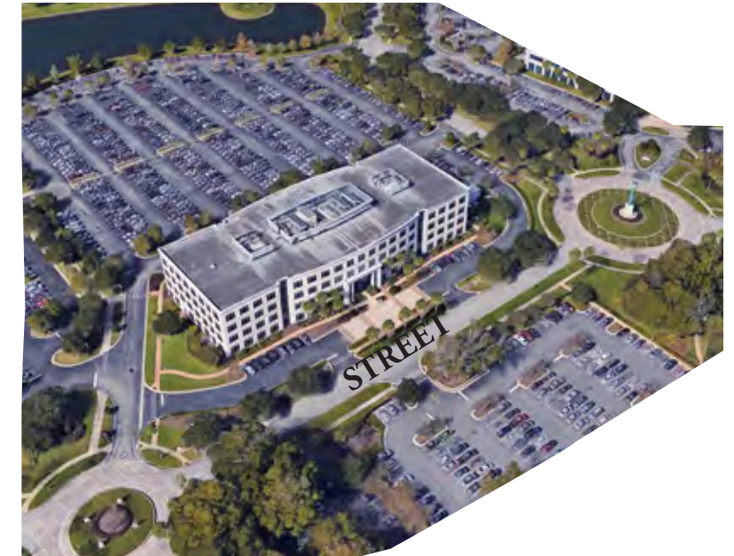
Example office building with limited parking between building and street and main parking field behind building
