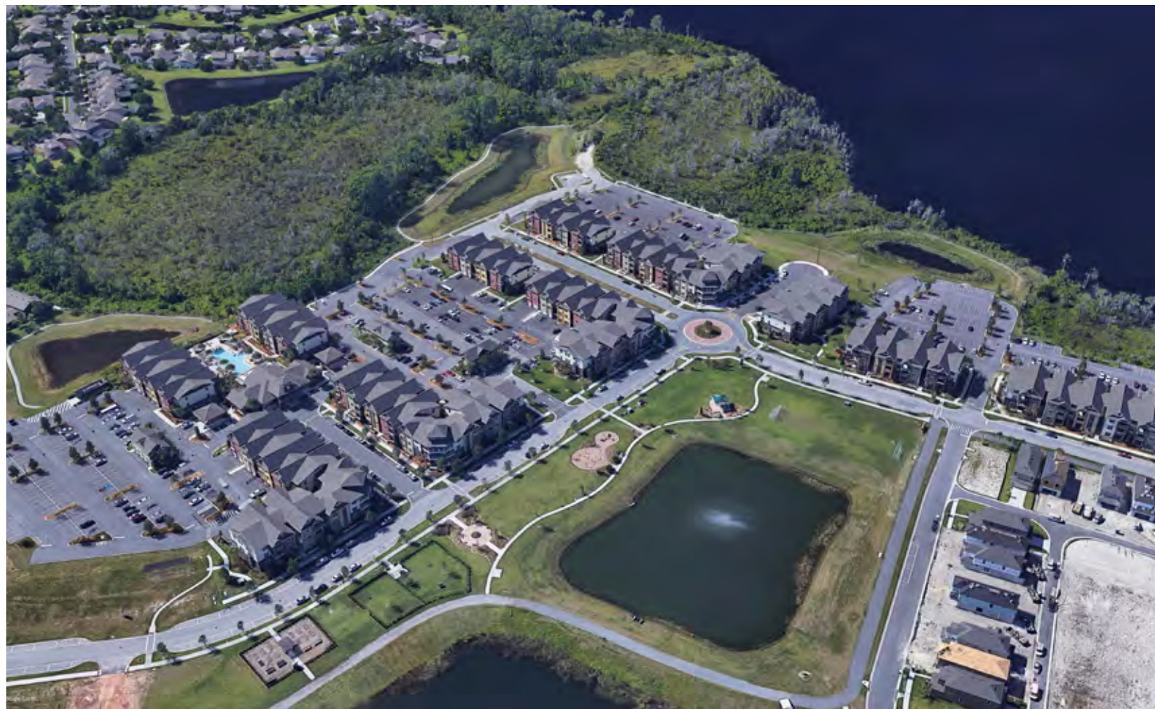
Example: Buildings are located at edge of sidewalk to spatially define the public realm. Parking is located at center of block where its impact on surrounding pedestrian areas is minimized.
