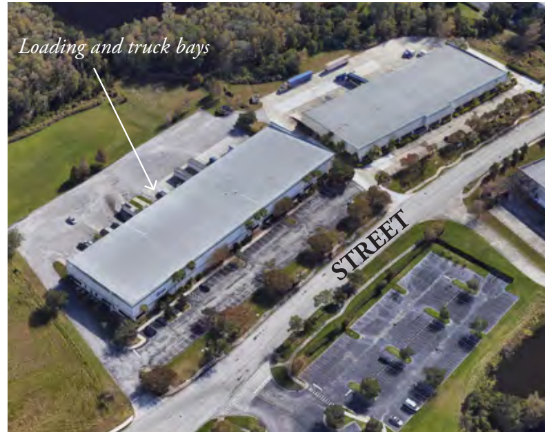
Example industrial building site configuration, with loading oriented away from street and limited parking in front of building
