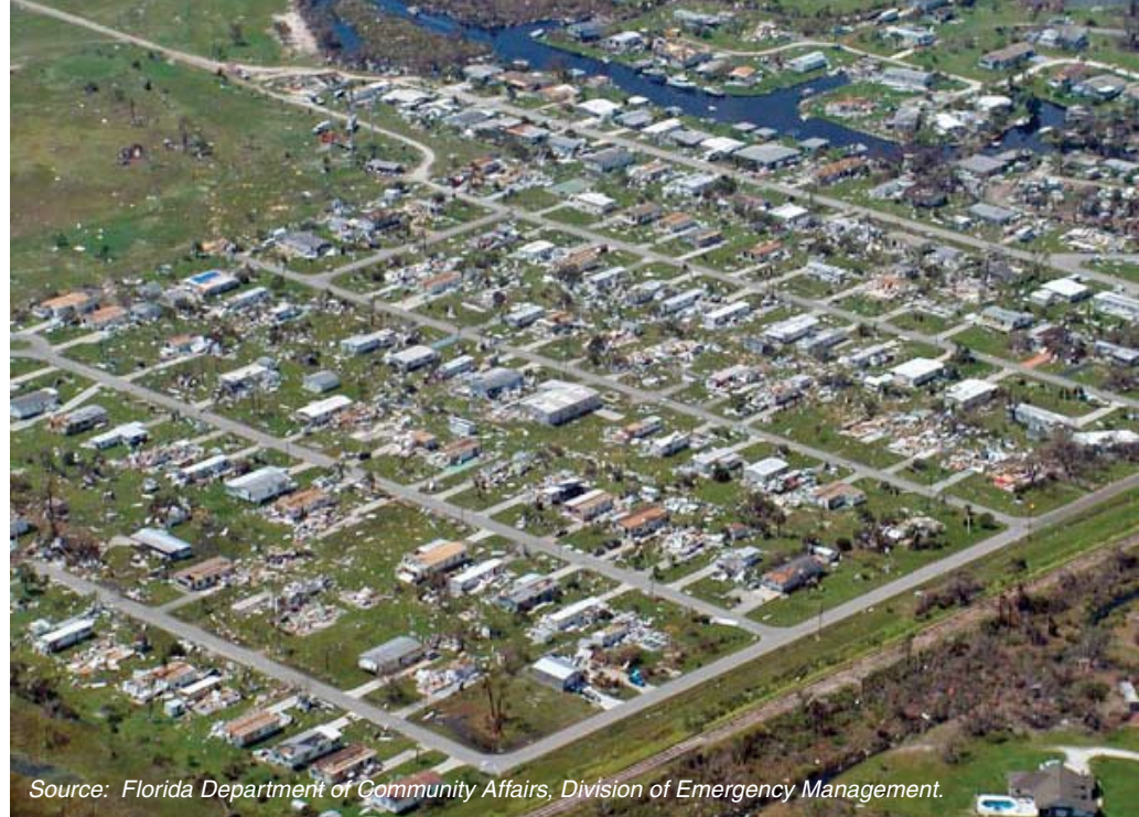
Figure 5.10: Mobile home wind damage from Hurricane Charley.
